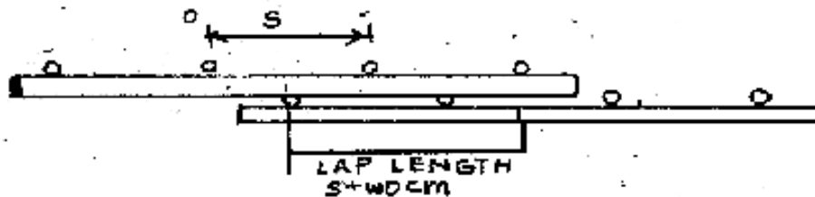
FIG - 3 : LAP SPLICING OF WELDED WIRE FABRICS
